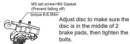
Adjust disc to make sure the disc is in the middle of 2 brake pads, then tighten the bolts.
