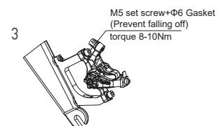
3. Adjust caliper to make sure the disc is in the middle of 2 brakepads, then fix the brake pads.
