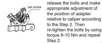
release the bolts and make appropriate adjustment of the position of adapter relative to caliper according to the Step 2. Then re-tighten the bolts by using torque 8-10 Nm and repeat Step 2.
